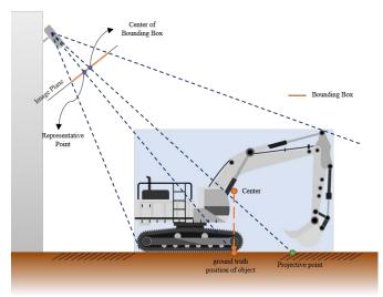
Fig. 1 The projective point of center of the bounding box
